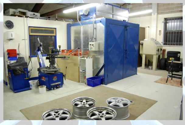
Our new facility includes a newly commissioned Industrial Oven which will be used for powder coating and curing. This allows us to recoat many sets of wheels in a day as well as producing a high quality long lasting finish for longevity.
